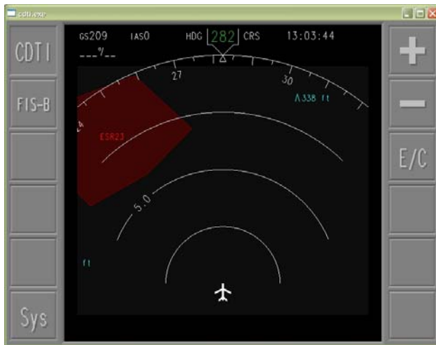
Aircraft passing activated Temporary Segregated Area (TSA), from D-AIM test flight, autumn 2008
