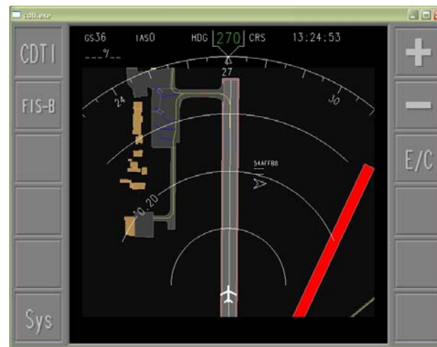
Aircraft landing on RWY 09/27 at Norrköping Airport, EFB showing RWY 11/29 Closure, from D-AIM test flight, autumn 2008
