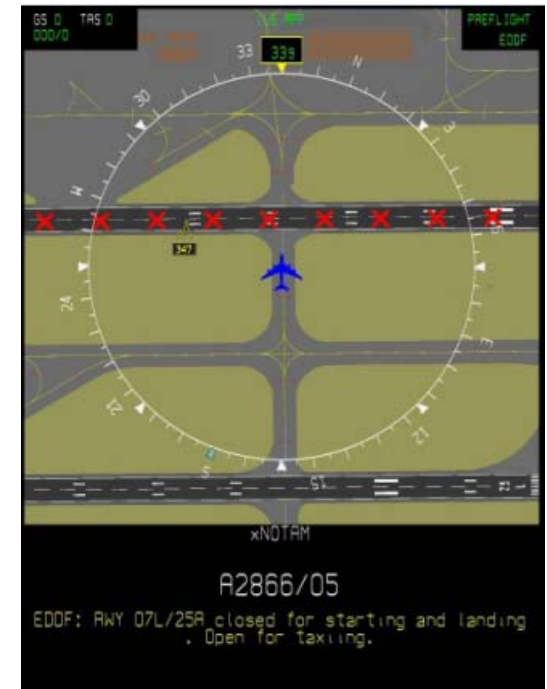
Picture from Digital NOTAM simulation performed by Technical University of Darmstadt in 2006
